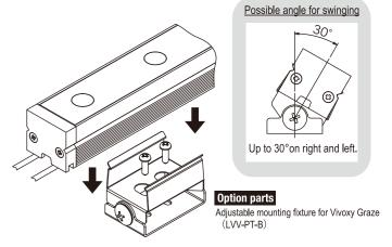
Fixed by screw (commercially available) (Screw hole 3.5mm×7mm.) Recommended screw: pan head screw M3
