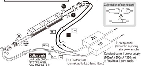
LED will be damaged immediately, if the fixtures are connected are on connected.
