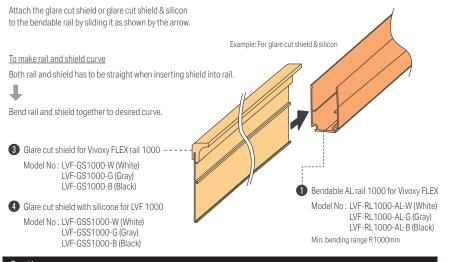
Glare cut shield, Glare cut shield & silicon length for each LED fixture length, The recommended length of installations is as follows.
