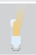
Bendable glare cut shield with silicon can be covered LED half to avoiding unexpected light spill, glare, light pollution for exterior
