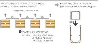
When inserting the LED fixture into the mounting parts, do not press with force using fingers or a tool, it may cause damages
