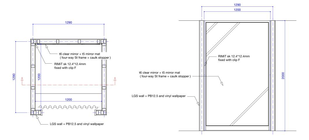
Horizontal cross section detail drawing S=1:2
