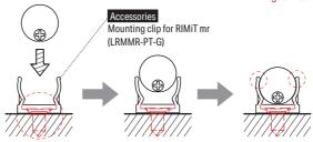
Fix the Mounting clip with screw supplied by (Recommended: Flat head screw M3)
