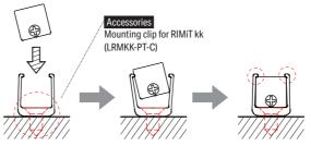
Fix the Mounting clip with screw supplied by (Recommended: Flat head screw M3)
