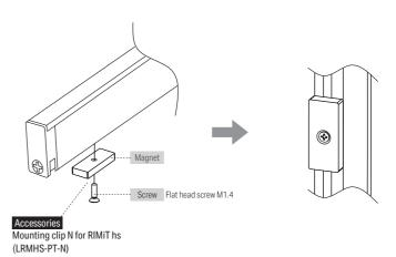
Please make sure that the flat screw is properly aligned and flush with the surface
