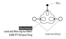
Attach the clip to the wire and insert the adjusted lead wire into the clip to bundle the wire and lead wire together.
