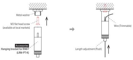
Attach the washers of the hanging bracket to the luminaire at both ends (2 poiints at each end) with screws (recommended: flat head screw M3 available at local markets). Secure the hanging bracket by rotating its body to lock it firmly in position.
