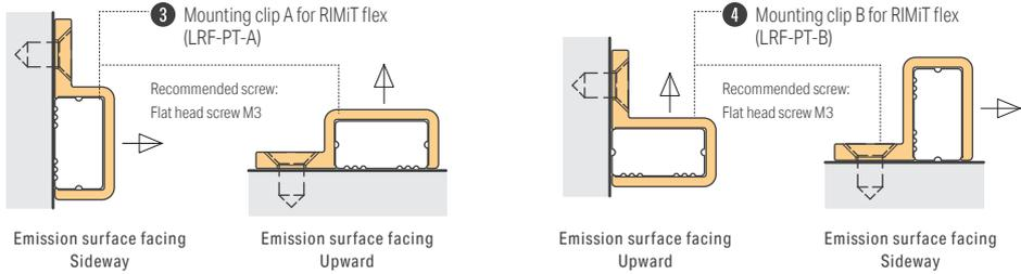
\* If any section of the LED fixture sags or deforms, please use more clips to secure the fixture.
