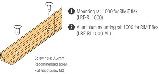
For upward installation
