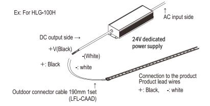
Always waterproof the wiring connections.
