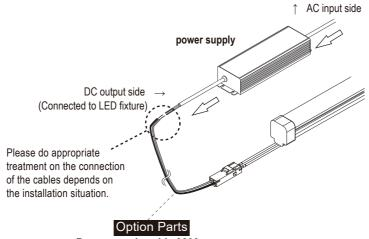
Power supply cable 3000mm for SL connector (CAD-3000-MCNN-I) +: Black -: White
