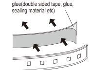
Always waterproof the wiring connections.
