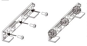
Installing clips should be set to the installation spot with shop-bought screws (pan head screws M3). (Recommended pitch under 380 mm, at least 3 per meter)
