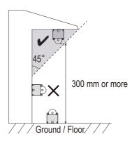
When using EFRO in semi-outdoor, it must be installed with the aluminum rail for EFRO. Please installed the LED fixture and the cable within the range of 45° eaves of the roof amd 300 mm or more away from the ground or the floor. Pleasedo not install the LED fixture and cables in the follow place:
